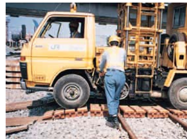
Zufahrtsrampe Carry-in base for High Rail Car
