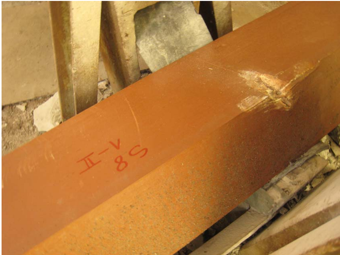
View of sleeper S8 after the second impact in derailment test I.
