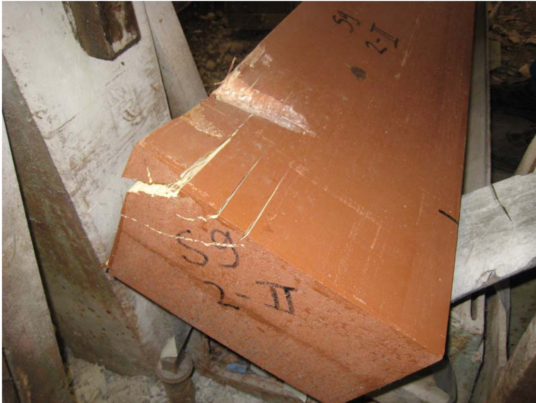
Caused by the homogeneous structure of the synthetic sleeper the derailment test shows clear and reproducible results.
