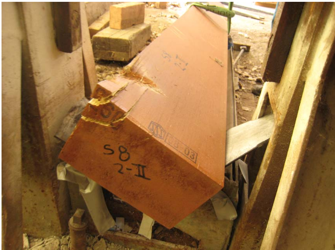
Wedge-shaped cutout of sleeper S8 derailment test II.
