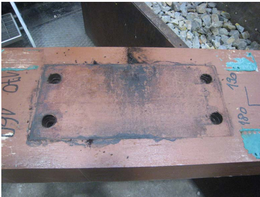
Permanent deformation of 0.3 to 0.7 mm on the sleeper surface after fatigue test (3.0 Million + 1.28 Million load cycles).
