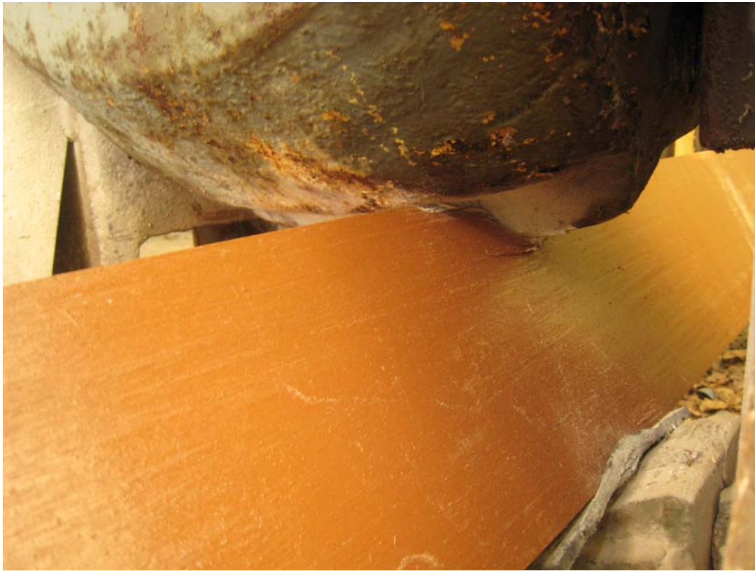
The tup with a wheel-flange shaped blade penetrates into the sleeper edge in a proper way. The damage is limited to a small area near impact position.
