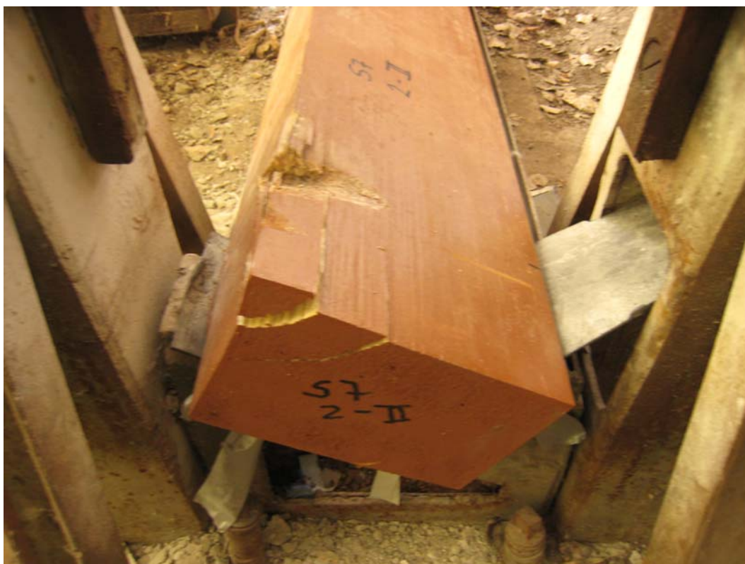
Wedge-shaped cutout after second impact in derailment test II.
