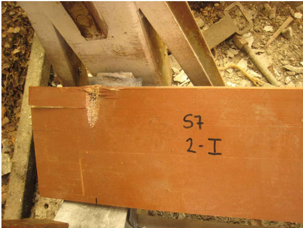
By derailment test II (impact on fieldside of the rail, 15 cm distance from sleeper front end) a wedge-shaped cutout is removed from the sleeper.
